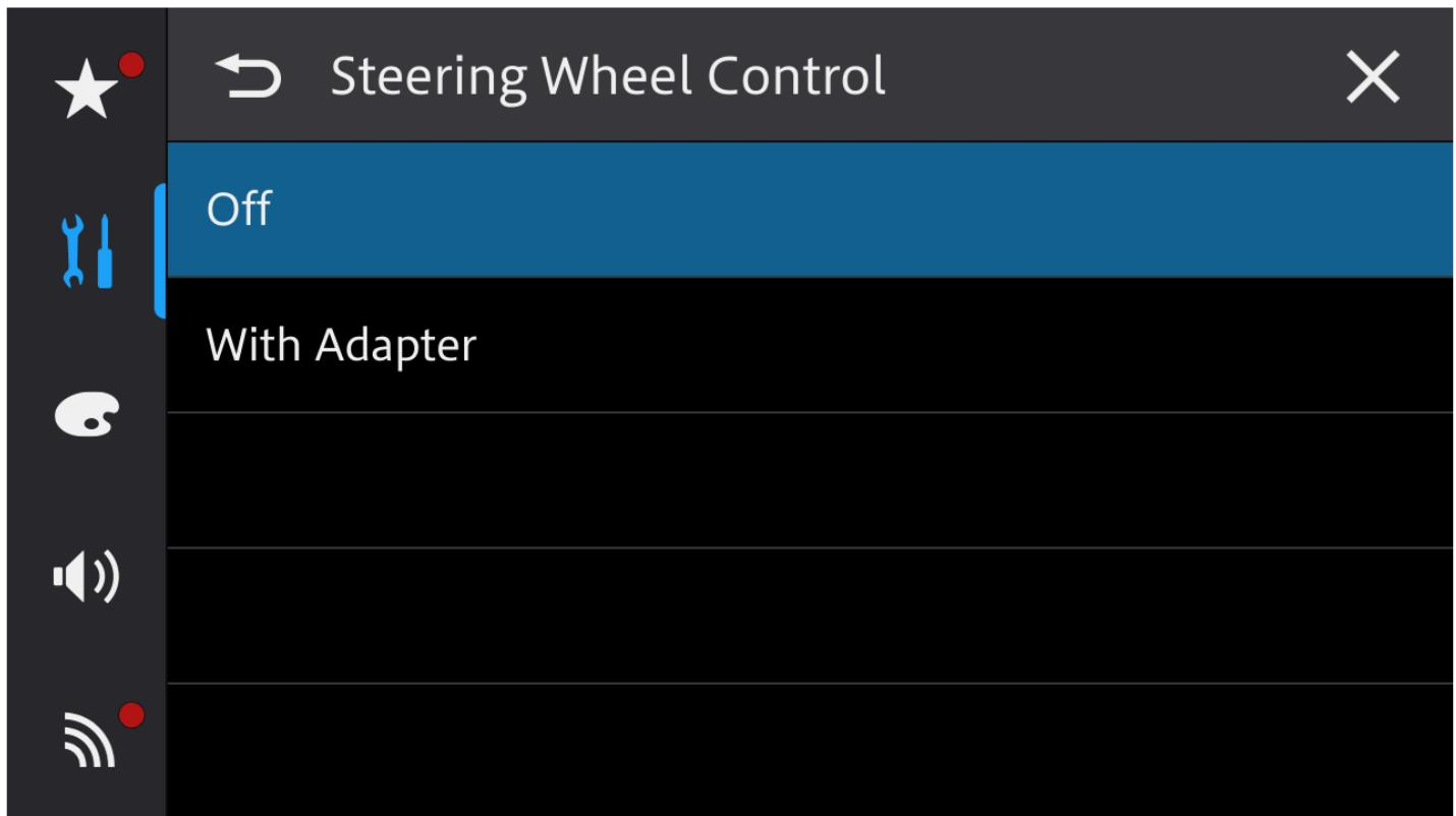
If the settings for the steering wheel controls are available in the Head unit, please choose the option “with adapter” to be able to use the steering wheel controls of the vehicle.
