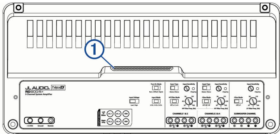
The LED light strip is solid blue when the amplifier is on and functioning normally.
