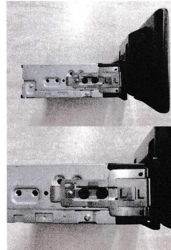
3) Now fix the left and right spring brackets on the silver box with the supplied screws, as shown in the pictures.
