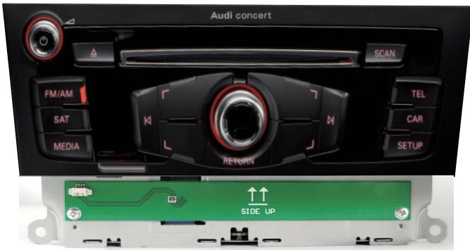
**NOTE!** Unplug the OEM FPC from main board of head unit and connect to the black connector above of provided board, then connect provided FPC cable to the OEM connector that just pulled out OEM FPC. Please pay attention to the direction of provided FPC board. (SIDE UP)
