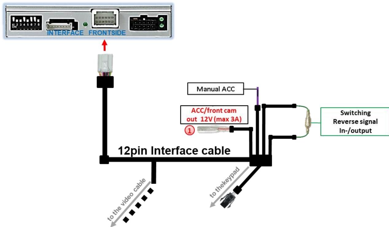
① The red power supply output **ACC/front cam out 12V (max 3A)** can be used to power an external source and has a different assignment depending on the position of dip switch 1 (of the black 8 dips):
