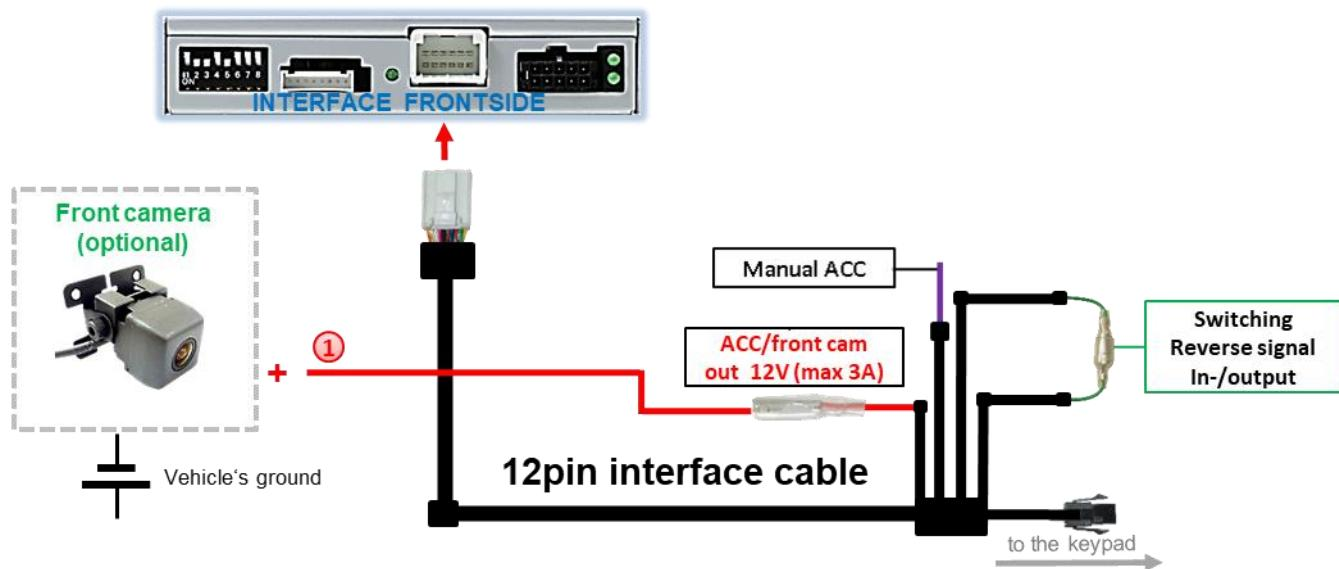
① The red power supply output **ACC/front cam out 12V (max 3A)** can be used to power a front camera. If Dip 1 is set to ON (black 8 dips), the power supply output gives +12V (max 3A) when reverse gear is engaged incl. 10 seconds delay after reverse gear is disengaged.
