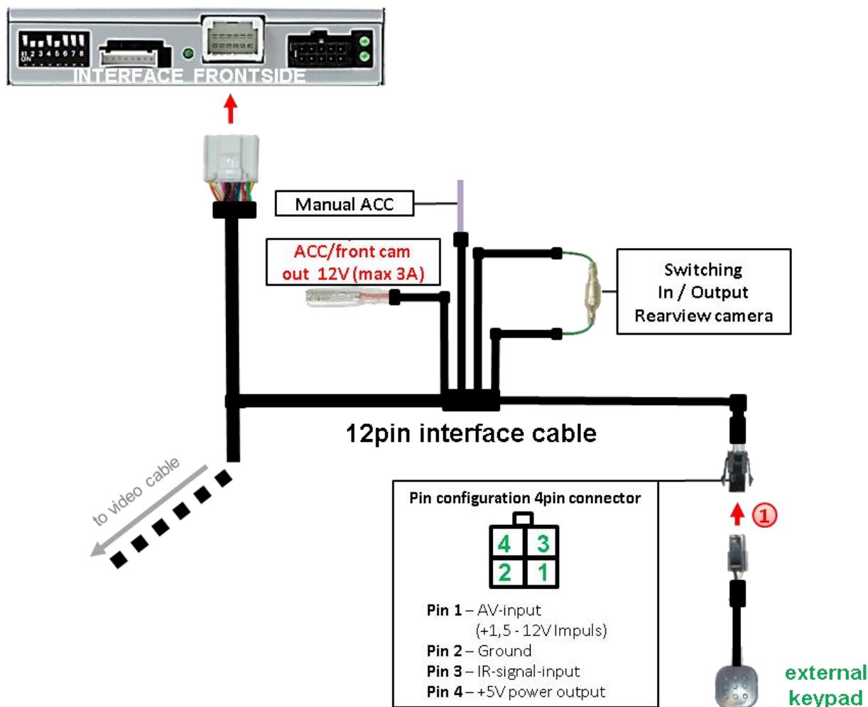
① Connect the keypad's female 4pin connector to the 12pin interface cable's male 4pin connector.
