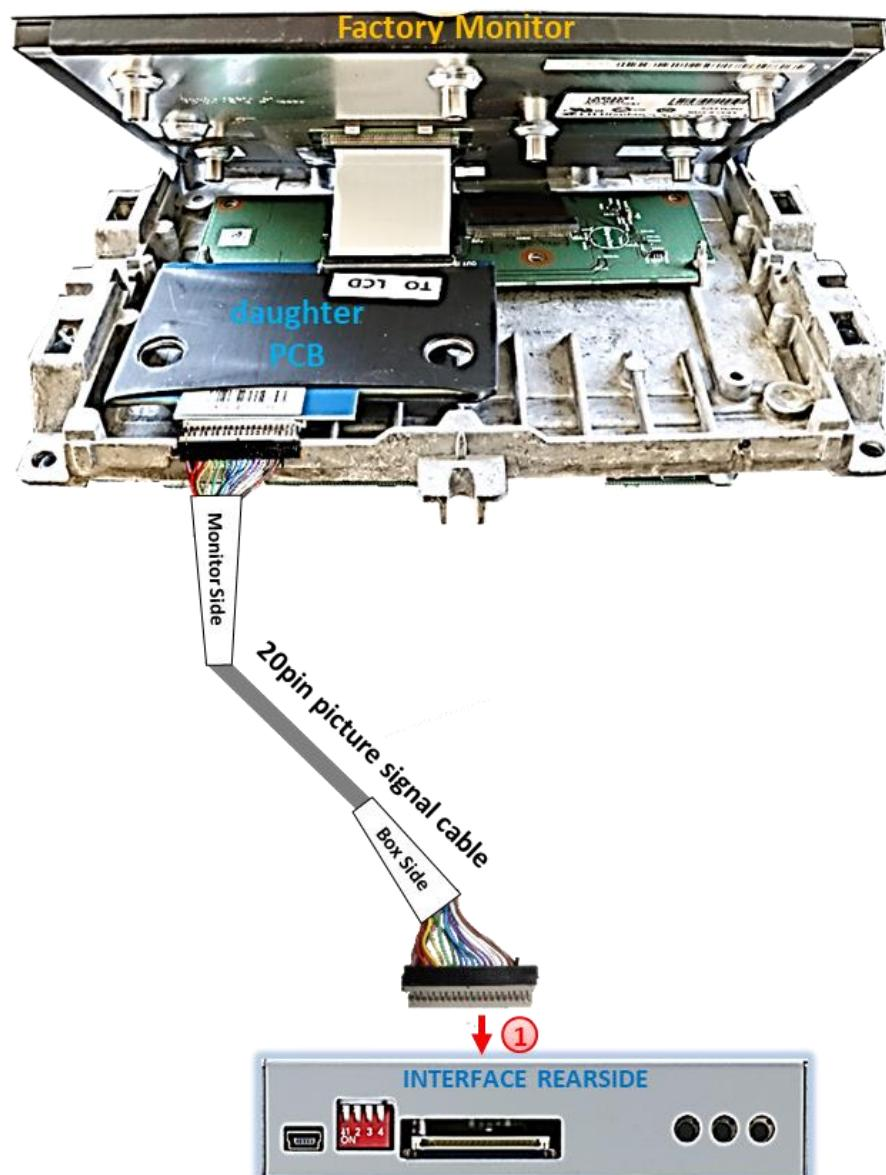
① Connect the opposite female 20pin connector of the pre-connected 20pin picture signal cable to the male 20pin connector of the video interface.
