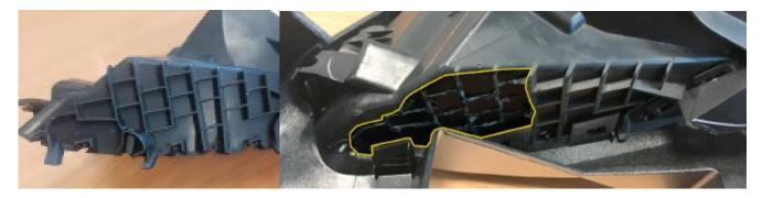
Next, Remove the screw clip circled in Figure 3 (Below)
