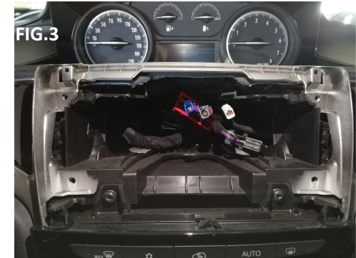
Remove the n.4 OEM screws where indicated (Image Fig.2). The OEM screws will be necessary to fix the Aftermarket kit. After removing OEM brackets and screws the dashboard will be as Image Fig.3
