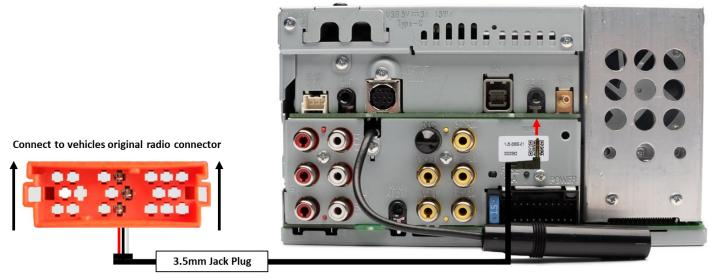
Connect the 3.5mm jack plug to the back of the Kenwood (Labelled REMO)
