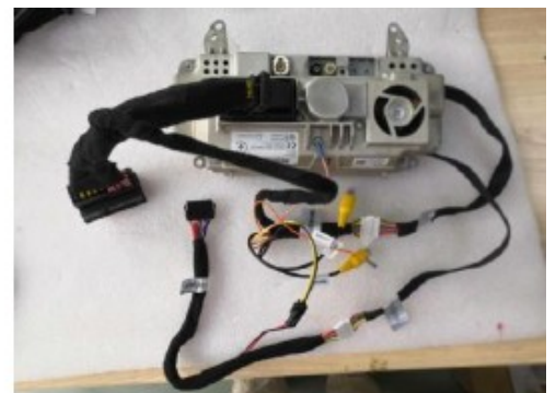
Refit back cover and connect new power cables
