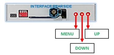
The picture settings are adjusted by the 3 buttons on the video-interface. Press the MENU button to open the OSD settings menu. To switch to the next menu item, pressing UP and DOWN will change the selected value. The buttons are embedded in the housing to avoid accidental changes during or after installation. The picture settings have to be done separately for AV1, AV2 and CAM while the corresponding input is selected and visible on the monitor.
