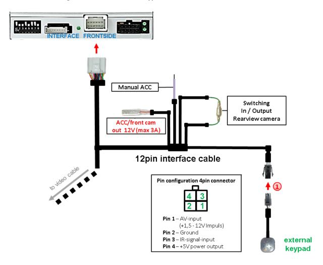
1 Connect the female 4pin connector of the keypad to the male 4pin connector of the 20pin interface cable.
