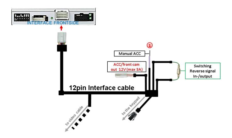
If, after connecting the PNP harness, no interface LED lightens up while the ignition is turned on, the single purple coloured wire Manual ACC of the 12pin interface cable has to be connected additionately to S-contact terminal 86s +12V (e.g. glove compartment illumination).
