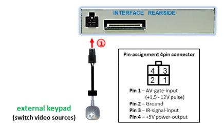
Onnect the keypad's female 4pin connector to the male 4pin connector of the video-interface.
