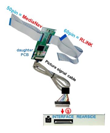
Onnect the female 20pin connector of the daughter PCB to the male20pin connector of the picture signal cable and connect the second male 20pin connector opposite the cable to the female 20pin connector of the interface. Take care for installing the cable in the right direction as both connectors seem to be identical. (Take notice of the wire's caption "MONITOR SIDE" and "BOX SIDE"
