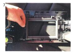
7 Install the supplied facia plate on the back of the previously removed original plastic panel as shown in the picture.
