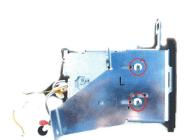
5 Tighten the 4 supplied screws (2 per side) to match the brackets with the body of the radio .
