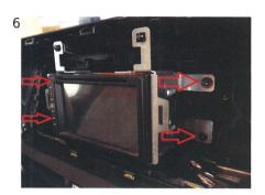
6 Connect all cables, verify the proper functioning of the system, install the radio in the radio tunnel and fix the 4 supplied screws as shown in picture.
