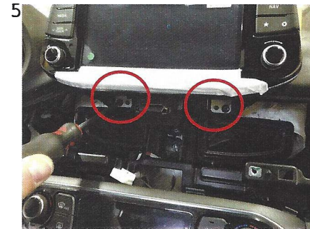
5 Remove and save the two screws and the original radio unit from their position.
