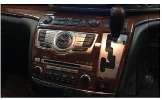
The original head unit can be hidden in the space that is filled by the storage box below the radio. The storage box will need to be modified to hold the head unit and will not be usable for storage any more.
