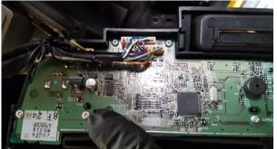
Connect the 20 pin female plug to the cars original wiring and the 20 pin male plug to the old head unit.
