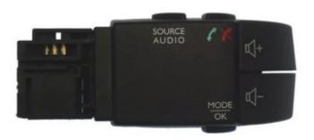
The interface is designed to be used with the above stalk paddle. The SOURCE AUDIO button will change source, the phone button will answer calls with a short press and reject with a long press. The volume buttons increase and decrease volume, the MODE OK button will skip through radio presets and the scroll wheel on the back of the paddle skips tracks forward and back.
