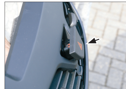
8. Place hazard light switch onto new 2-DIN fascia plate
