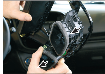
6. Unclip and remove air vents from OEM panel
