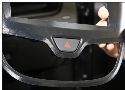
6. Place hazard light switch onto new 2-DIN fascia plate
