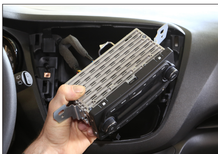
4. Unplug all connectors Remove OEM head unit
