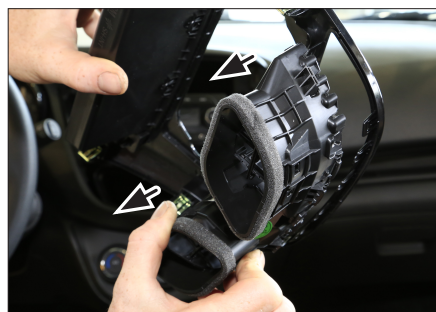
7. Unclip and remove air vents from OEM panel
