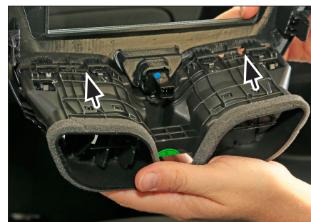
8. Place air vents onto new 2-DIN fascia plate
