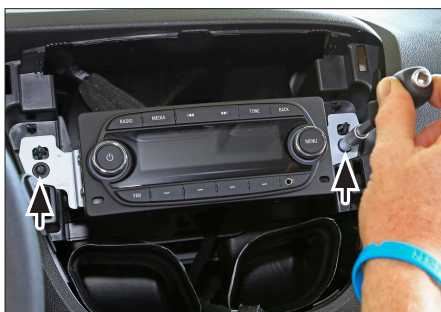
3. Remove 2 screws of OEM head unit (see arrows)
