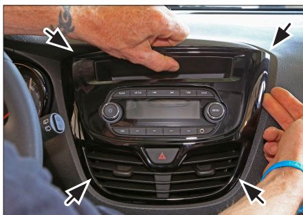
2. Unclip OEM panel Unplug hazard light switch and remove OEM panel
