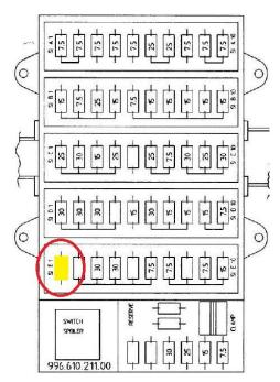
In the spare slot on the fuse holder, insert the same specification fuse that was originally in the slot in the fuse box that it has been connected to.
