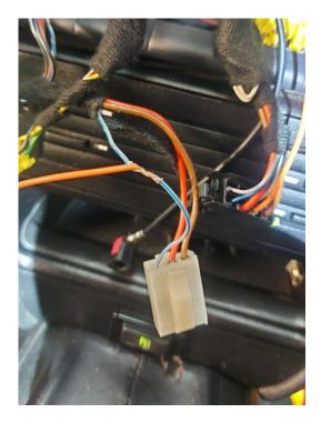
The purple wire for the reverse feed is for switching to an aftermarket reverse camera if fitted when the vehicle is put into reverse gear.
