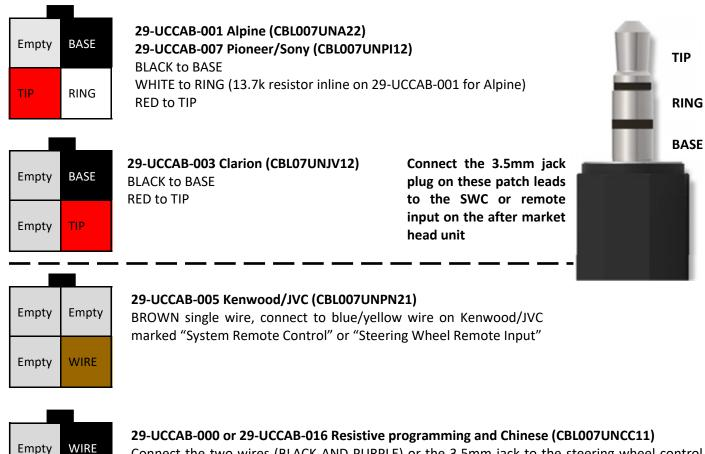
Connect the two wires (BLACK AND PURPLE) or the 3.5mm jack to the steering wheel control inputs on the head unit. If head unit uses 2 wire system then connect to SWC1 and SWC Ground or KEY1 and KEY Ground wires. The steering wheel controls will need to be programmed into the head unit after setting the number of flashes. See overleaf.
