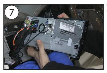
With the screws removed, the head unit and bracket assembly can be pulled partially out of the dash
