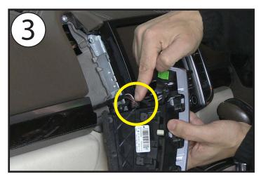
Once the vent has been released from the dash, disconnect the sensor connector and place the vent safely to one side for reassembly.
