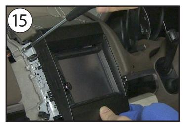
Once the stereo is in place, screw it into the dashboard using the four screws removed during Step 5
