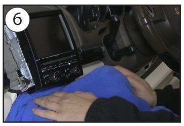
Ensure that the gear shifter/lower dash is covered by a suitable protective material to prevent scratching or damage for the next steps
