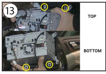
Screw the fascia panel onto the mounting brackets at the four points (two at the top and two at the bottom) at the back of the fascia panel using the four self-tapping screws provided with the kit.
