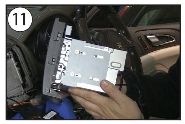
Screw the right and left mounting brackets onto the new head unit using the radio mounting screws provided
