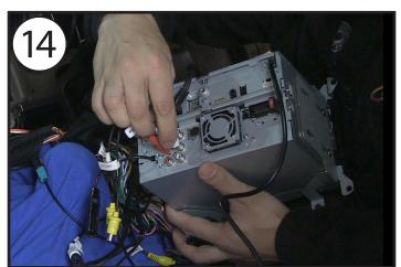
Make wiring connections from the vehicle side to the stereo and push the stereo into the dashboard being careful not to trap any wiring.
