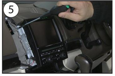
Remove the four Torx screws from around the head unit and safely store for reassembly.
