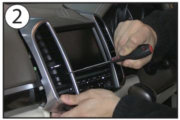
There are six clips that are currently engaged to hold the left-hand vent in place, two on the left and right, and one on the top and bottom. To disengage these clips, push a screwdriver or similar tool through the vent and push outwards to release each clip. Use a torch for a better view of the clips during this step.
