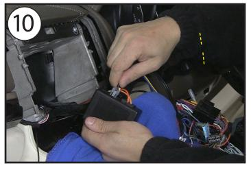
If installing a full kit, make the connections to any interfaces at the vehicle side. Please see the corresponding interface instruction manual for more information on making these connections
