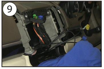
With the connections unplugged, the entire head unit and bracket assembly can be removed from the dashboard
