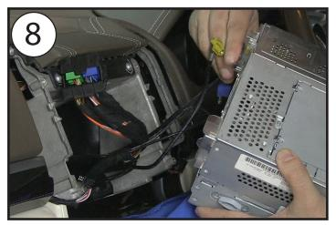
Next, ensure that all connections at the back of the head unit are disconnected
