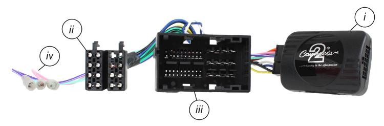
i. Interface Box ii. Male ISO Connector (16 Pin) iii. Fiat Vehicle Connector iv. Flying Wires (Green - Park Brake / Pink - Speed Pulse / Purple/White - Reverse Gear)
