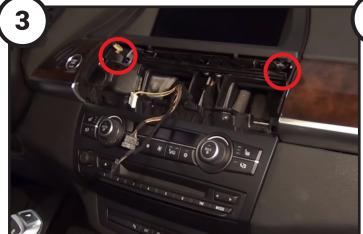
Remove the two screws securing the upper OEM display. Disconnect and remove the display.
