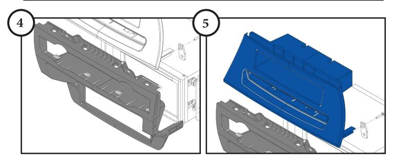
Surround the head unit with the lower panel and lock into place using the clips retained from the OEM panel and the OEM screws.
