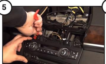
Use a panel removal tool to remove the lower fascia panel/ Remove the two screws securing the OEM head unit in climate control assembly. Disconnect and remove the panel.
