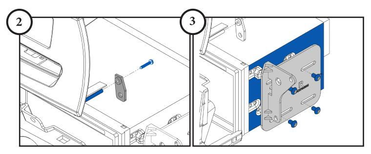
Screw each relocation mount into place at the bottom right Screw the right and left brackets to the sides of the after-and left corners of the upper panel using the x2 Pozi Pan market head unit using the Hexsocket screws included screws included with the kit
