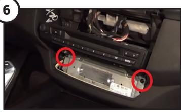
place. Disconnect and remove the head unit.
