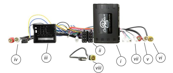
i. Interface Box ii. ISO Connector (16 Pin) iii. Quadlock Connector (40 Pin) iv. \*RCA Amplifier (Red/White)
