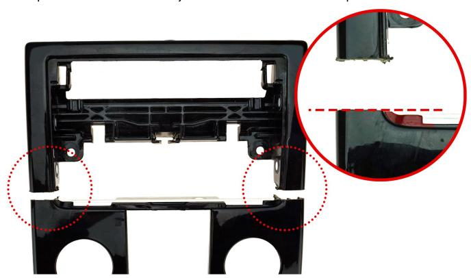
2. The original panel will need to be cut. See highlighted section. Cut the centre panel in line with the highlighted tab just above the bottom of the opening on each side.
