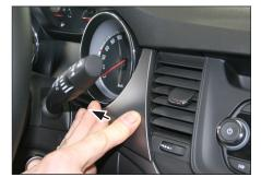
Remove panel cover between steering wheel and air vent (see arrows)
