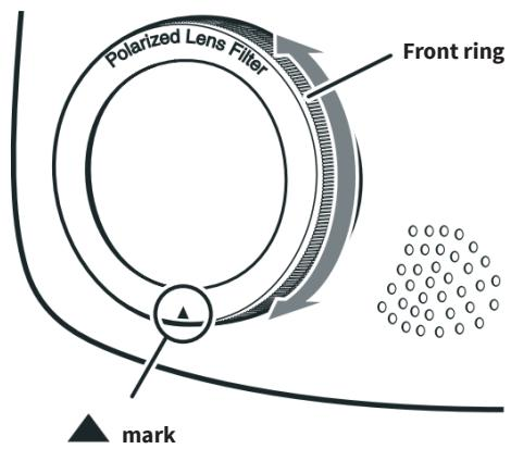
④ Place a white piece of paper on the dashboard to make the set up easier. Slowly rotate the ring on the front side and adjust it to a position where you can see the reflection effect of the paper reduced.
