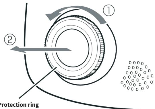
② Turn the ring on the back side and tighten it firmly. Be careful not to overtighten.
