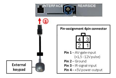
1 Connect the 4pin female connector of the external keypad to the male 4pin connector of the video interface.
