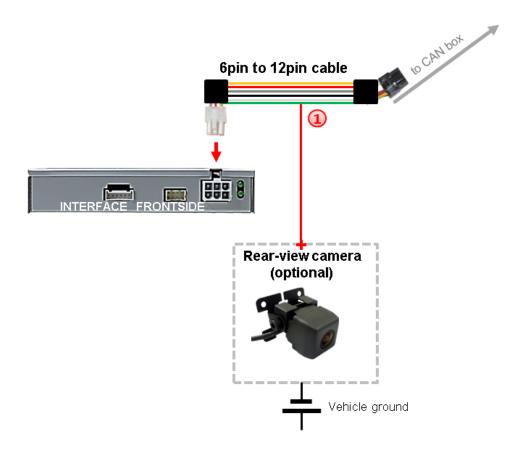
Additionally, the +12V (max. 500mA) power supply for the rear-view camera can be taken from the green wire of the 6pin to 12pin cable.
