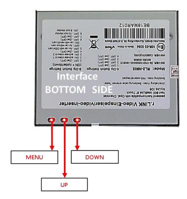
The picture settings are adjusted by the 3 buttons on the video-interface. Press the MENU button to open the OSD settings menu or to switch to the next menu item. Press UP and DOWN changes the selected value. The buttons are embedded in the housing to avoid accidental changes during or after the installation. Picture settings have to be done separately for AV1, AV2 and CAMERA-IN while the corresponding input is selected and visible on the monitor.
