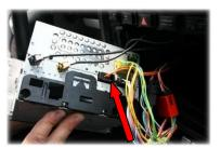
Connect black wire to ground and red wire to permanent +12V. Isolate blue wire.
