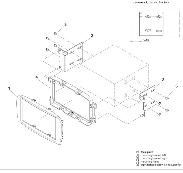
An appropriate installation in observance of these operating instructions is necessary. Please make sure the wiring is arranged so it is not bended or crimped due to the risk of cable break. Make sure that all connections are correct. Route the cable away from moving parts, do not allow the cable to be entangled, pinched or damaged in any way.
