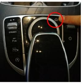
For Automatic Parking Function, press HOME button for 2 seconds to exit 360 and adjust to automatic parking
