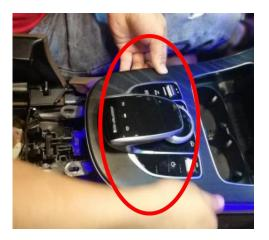
Lift away the centre console and the relevant cables
