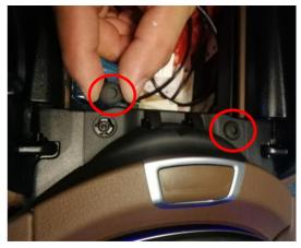
Remove the two rubber screw covers from around the centre console
