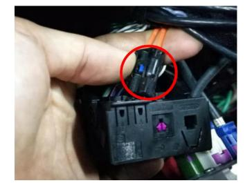
Remove the OEM Quadlock and move the Fiberoptic plug to the new quadlock on the interface
