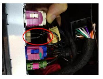
Unplug the LVDS Connector and connect the new LVDS IN connector to the head unit. Connect the original LVDS connector to the LVDS OUT connector from the in-
