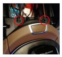
Remove the two screws and lift away the plastic facia cover
