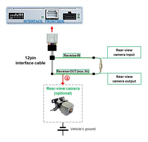
The 12 V power supply for the rear-view camera (max 3A) has to be taken from the green wire of the 20pin cable to avoid an unnecessary permanent power supply to the camera electronic.
