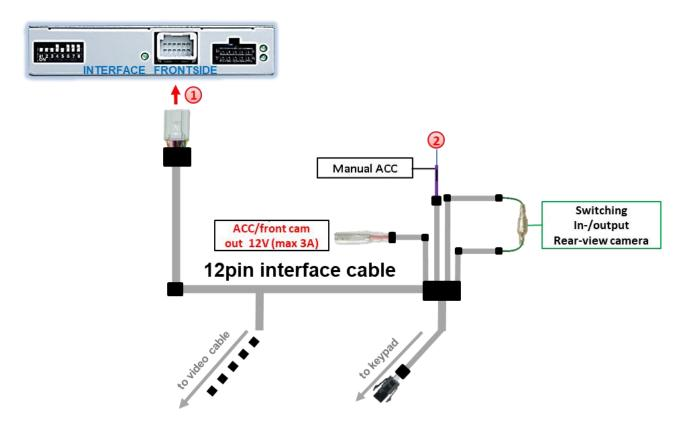
Connect the female 12pin connector of the 12pin interface cable to the male 12pin connector of the video interface.
