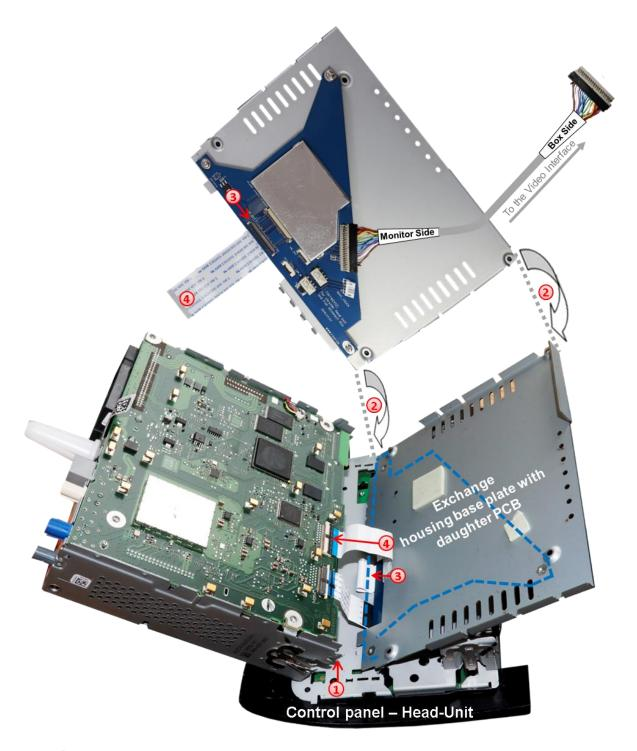
Clip out the head-unit housing at the head-unit control panel and fold it to the side, like shown in the picture above. Note: The connected ribbon cables have to be handled with care to avoid each damage of the sensitive electrical inducters.
