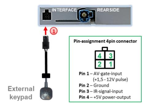
Onnect the 4pin female connector of the external keypad to the male 4pin connector of the video interface.
