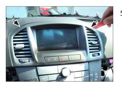
5. Unclip and remove OEM display
