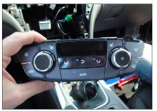
8. Remove air condition control unit from OEM panel
