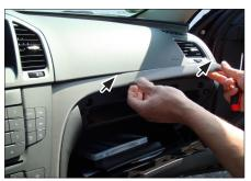
3. Unclip side panel (left) and remove it
