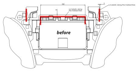
10. Cut plastic from dash board in order to clear space for the double DIN head unit (see lines in the drawing)
