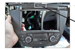
11. Mount air condition control unit to double DIN facia place
