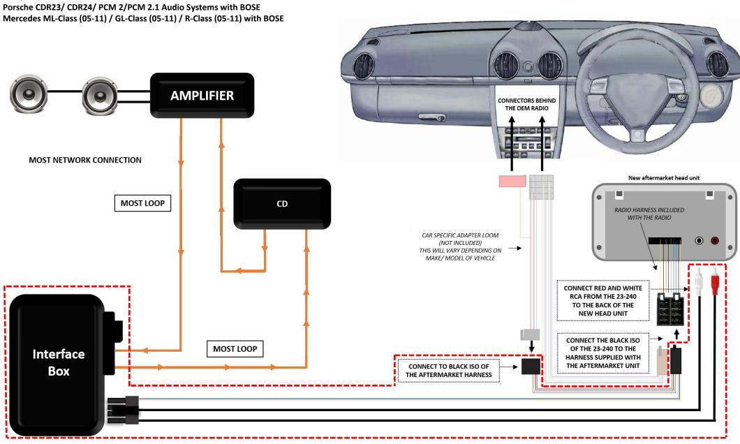
\*The Red Border indicates the 23-240 components and where to make necessary connections
