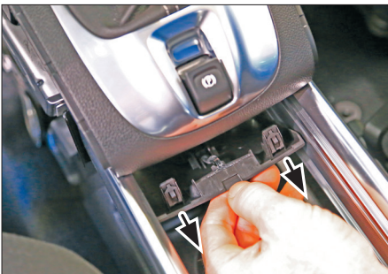
4. Unclip and remove panel under the gear box (see arrows)
