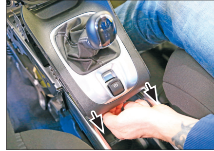
5. Pull gear box panel slightly into your direction (See arrows)
