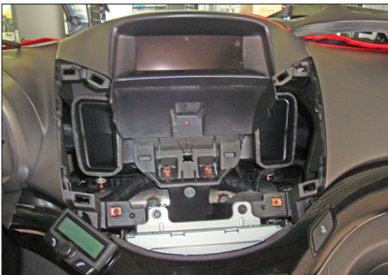
4. Dash board with removed panel
