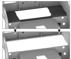
8. After cutting reinstall plastic frame into dashboard
