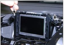
Remove two TX20 screws of 3. display **Remove display**
