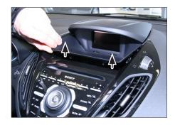
Unclip and remove 1. panel on top of B-MAX dashboard (see arrows)
