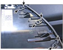
9. Remove air vents carefully (double clipped /see arrows) and air vent trim frames from OEM panel. Installation Manual Double DIN Kit silver/ piano black:
