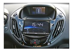
12. A new hazard light switch by Ford is required: part-no.: 1519127 Attach hazard light switch to new facia plate
