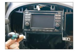
5. Remove screws of OEM head unit
