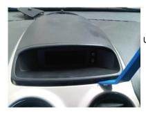
Using a panel removal tool, unclip and lift off the display cover.
