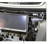
Connect all required circuit points. Place Double-DIN head unit on dash board Fix it with 4 screws
