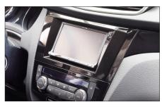
10. Put clips on the rear side of facia plate. Place facia plate on dash board
