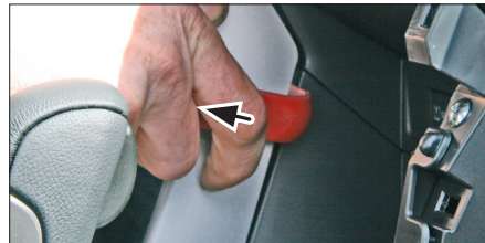
7. Remove deco panels on the left and right side
