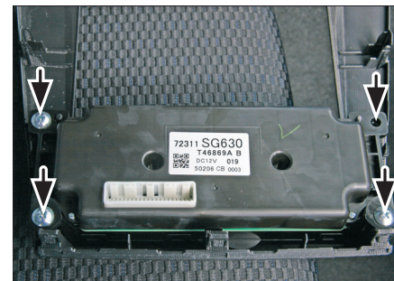
12. Mount climate control to new facia plate
