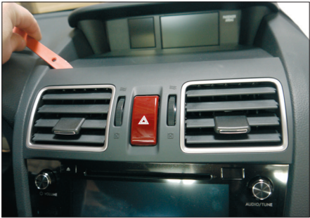
6. Unclip and remove air vents (unplug cables carefully)
