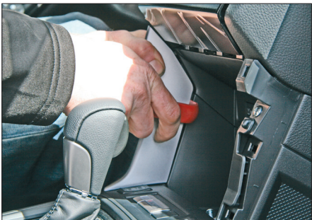
7. Remove deco panels on the left and right side
