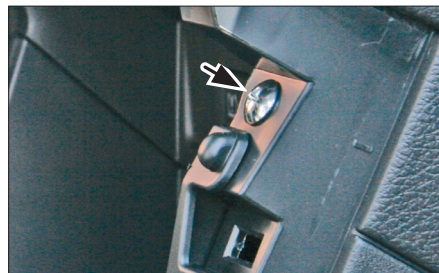
8. Remove screws (see arrows)
