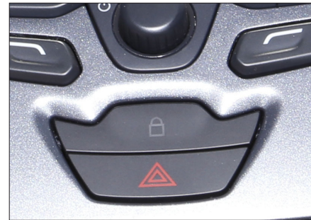
7. Depending on type of OEM head unit remove „HAZARD LIGHT SWITCH“ and „PASSENGER AIRBAG“ display
