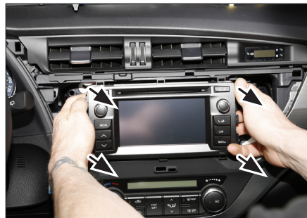
5. Remove OEM head unit by pulling it towards your direction (see arrows)
