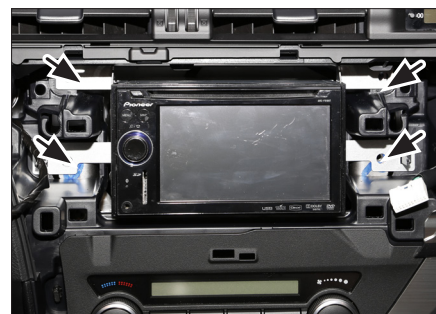
7. Connect all required circuit points place Double DIN head unit and fix it with 4 screws (see arrows)
