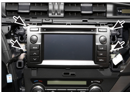
4. Remove 4 screws of OEM head unit
