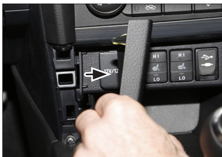
2. Remove plastic clips at left and right side beside climate control unit
