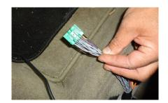
**7-**Remove the drivers side centre console side trim. Pull back carpet. Route the bypass cable wire from the amplifier (via the air duct and original speaker wiring) to the back of the facia.
