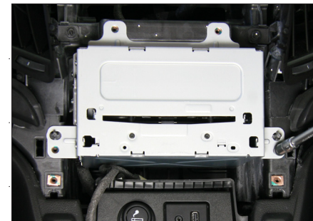
8. Remove screws of OEM head unit
