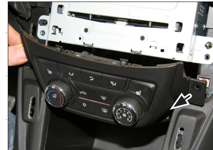
7. Remove screws of air condition control unit
