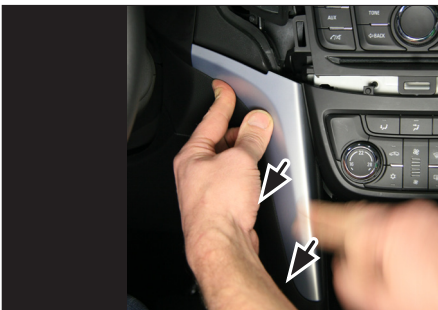
4. Unclip and remove left decor panel
