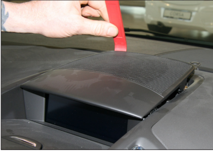
1. Unclip and remove top panel
