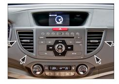
1. Unclip and remove air vents left and right side (see arrows)
