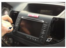
2. Remove screws of OEM head unit (see arrows)
