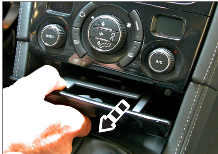
1. Remove lower tray under OEM head unit
