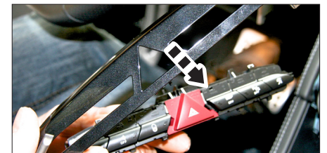
7. Remove top panel Remove buttons
