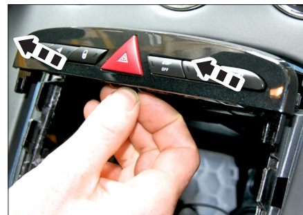
7. Remove top panel Remove buttons
