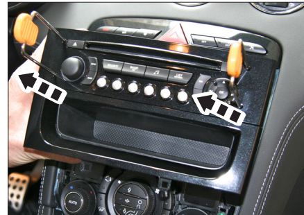
5. Remove OEM head unit
