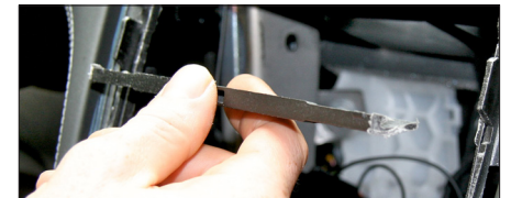
6. Cut away middle bar to clear space for double DIN head unit
