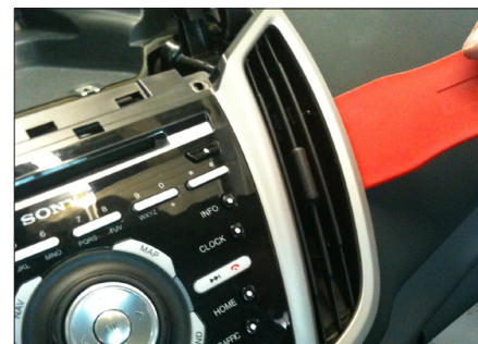
13. Unclip air vents Remove air vents
