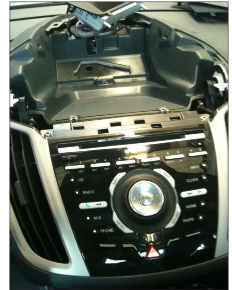
12. Remove screws on top of OEM head unit (left and right)
