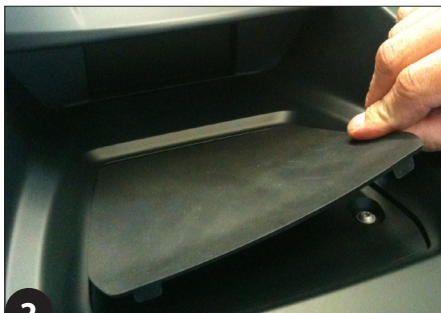
4. Unclip cover of center console
