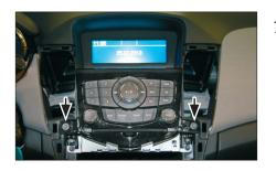
7. Remove screws of OEM radio (see arrows)
