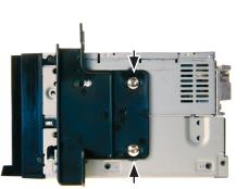
12. Mount the mounting brackets to the Double DIN head unit.
