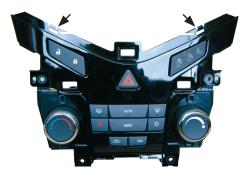
10. Cut out two edges from the OEM panel in order to clear space for Double DIN head unit (see arrows)
